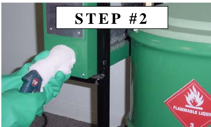
Cover with a rag, creating a seal around the pipe.
