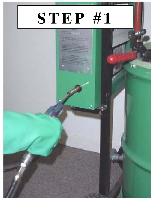
Insert air gun in the exhaust pipe.
