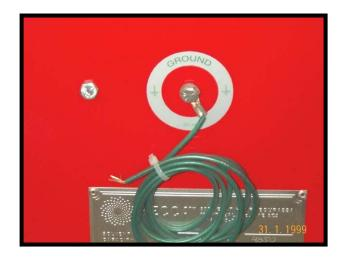
**<u>Step 2</u>**: The Spray Gun Cleaner must be grounded to your ground system.
