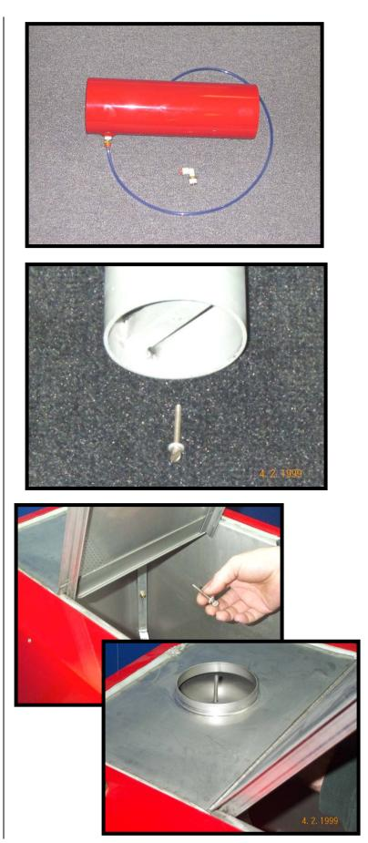
**<u>Step 4</u>**: Take the fume extractor cylinder kit and place it on the top of the unit.
